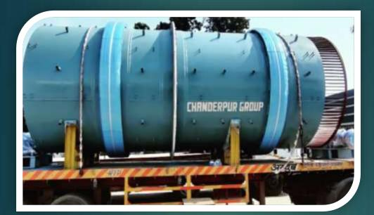
Rotary Granulator Steel Tyre Supported
